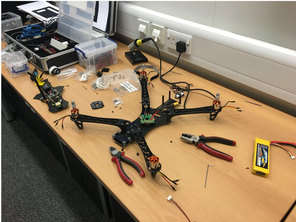
Figure 45 - Rebuilding the Spyda 500
