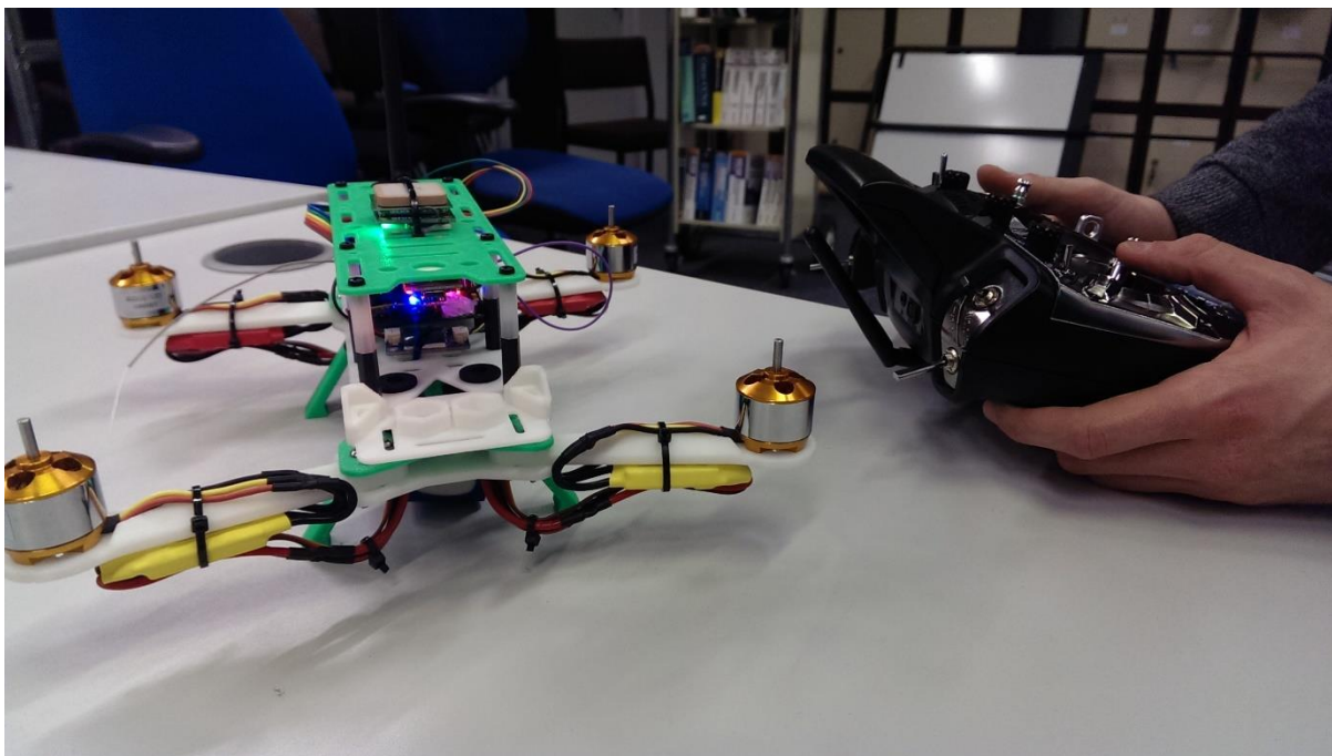
Figure 13 - Fully built MHQ2 without propellers during testing.
