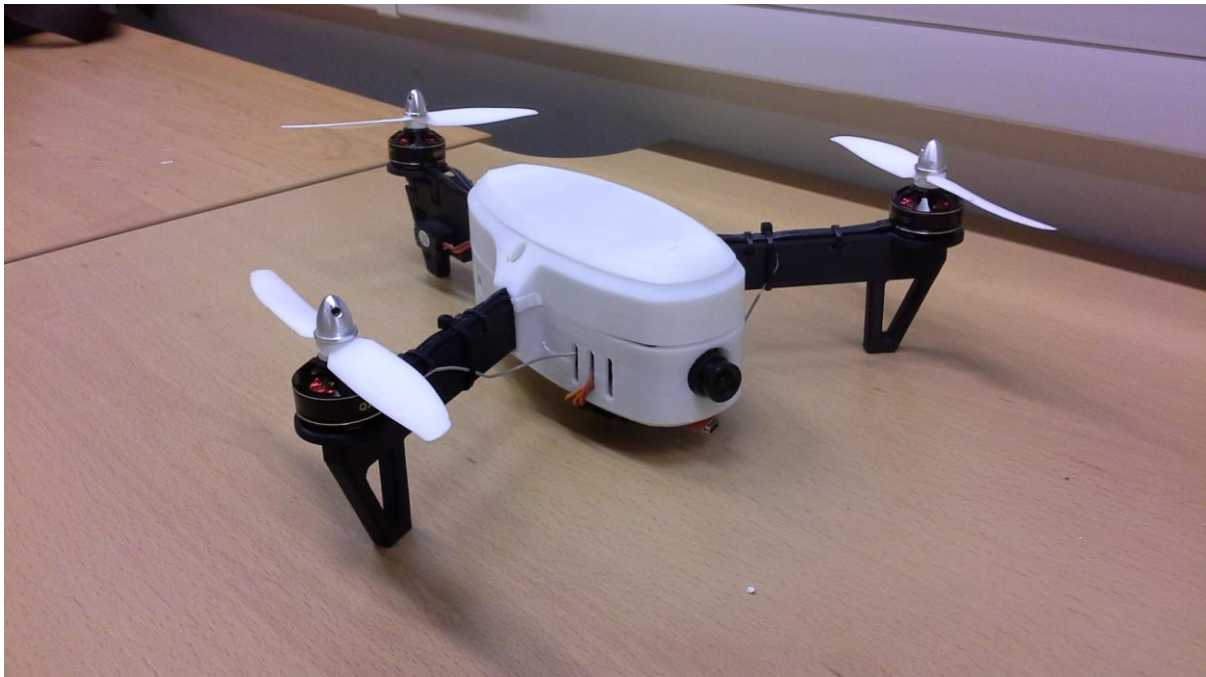
Figure 33 – 3D printed FPV tri-copter used for development of analogue video transmission
