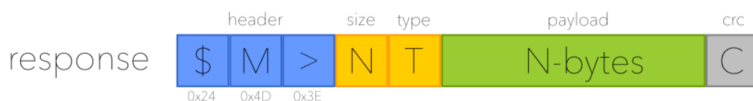
Figure 16 - Structure of an MSP response
