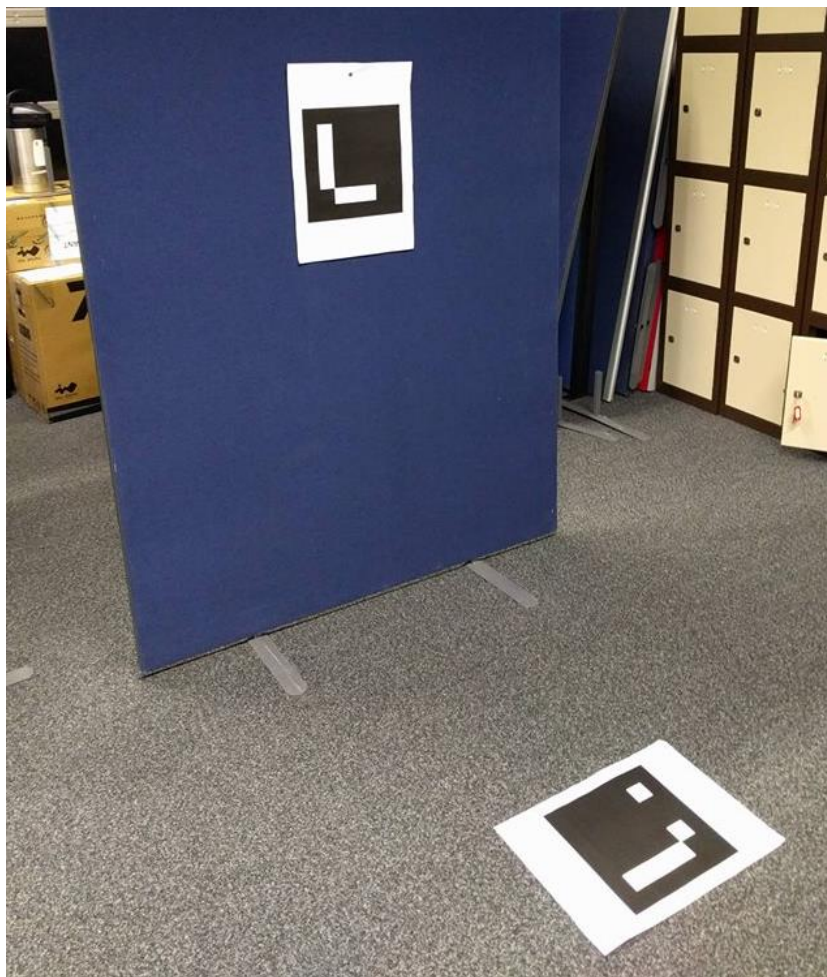
Figure 55 - Setup of Aruco markers used during testing with the multi-robot
