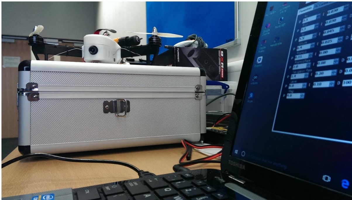
Figure 8 – Tuning the PIDs for the 3D printed tri-copter.
