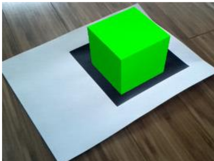
Figure 50 - Example of AR marker used to place virtual object in the real world
