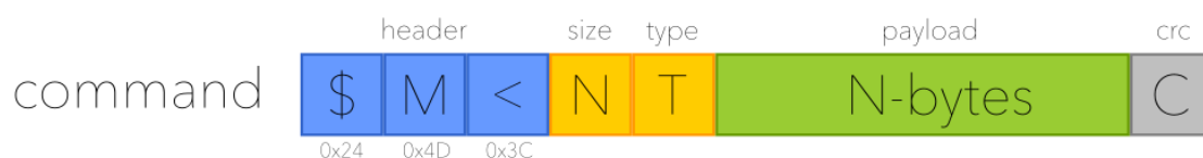
Figure 15 - Structure of an MSP command
