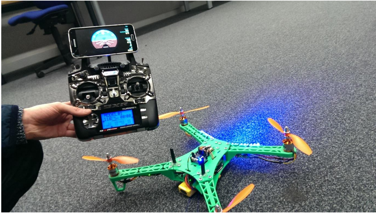
Figure 30 – Completed 3D printed Spyda 500 connected to smart phone for testing
